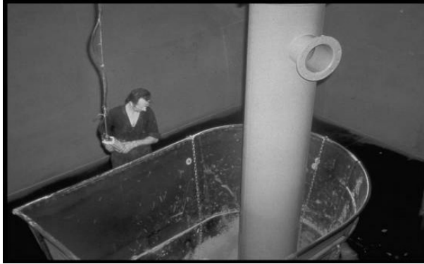
Fig. 2. Vertical fluid bed of polyamide 11
