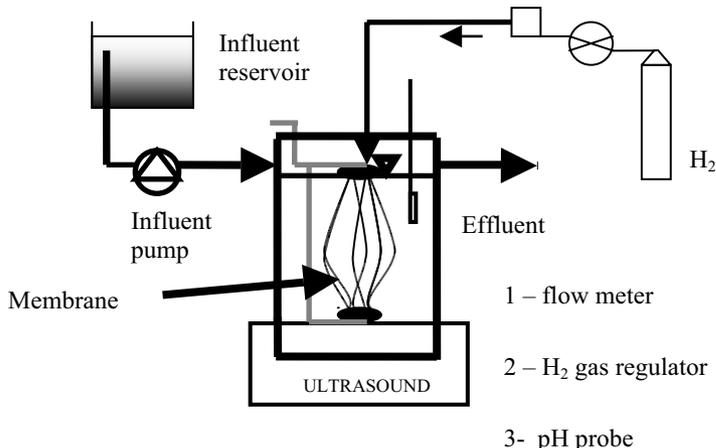
Fig. 1 Membrane biofilm reactor set – up
