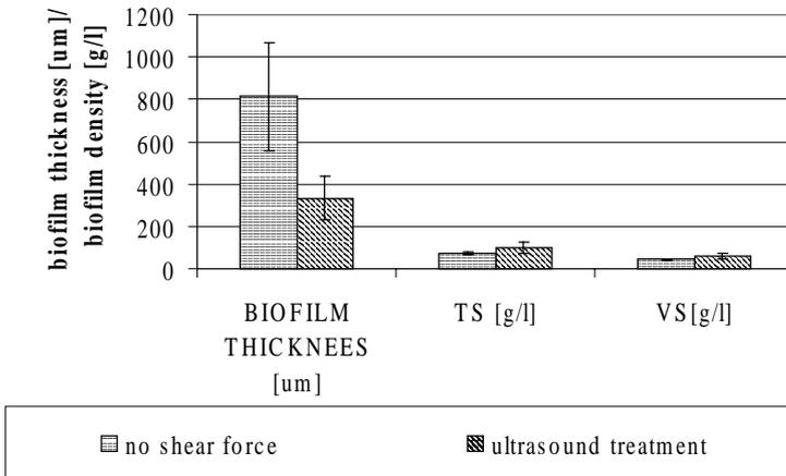
Fig. 2 Fluctuations in biofilm thickness and density in MBfR exposed to no shear force and ultrasound treatment
