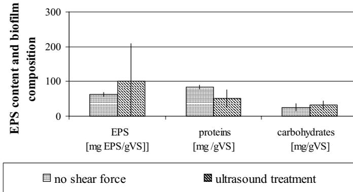
Fig. 3 Fluctuations in EPS, proteins and carbohydrates content in MBfR exposed to no shear force and ultrasound treatment
