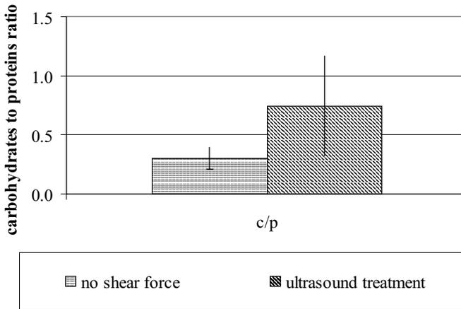
Fig. 4 Fluctuations in c/p ratio in MBfR exposed to no shear force and ultrasound treatment
