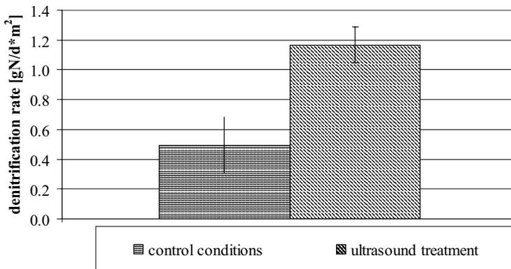
Fig. 6 Denitrification rates obtained in MBfR exposed to no shear force and ultrasound treatment
