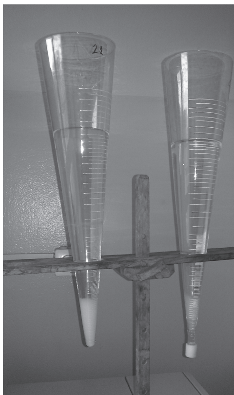
Rys. 3. Popłuczyny z filtrów P1 i P2 w lejach Imhoffa po 2 godzinach sedymentacji Fig. 3. The washings from filters P1 and P2 in Imhoff's funnels after two-hour process of sedimentation
